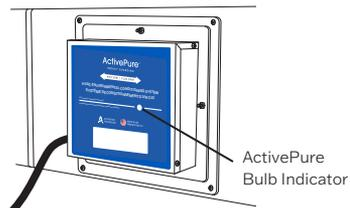
8. Re-install unit if removed from duct. Reconnect power and check for proper operation.
